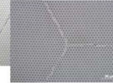
Photo of 6 μm pore, 63% open area, 60:1 L/d, C5
