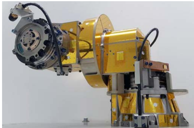
Gimbal developed by SENER for EUCLID
