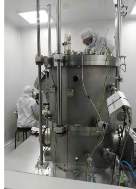
GOLD deposition chamber in an ISO-6 clean room
